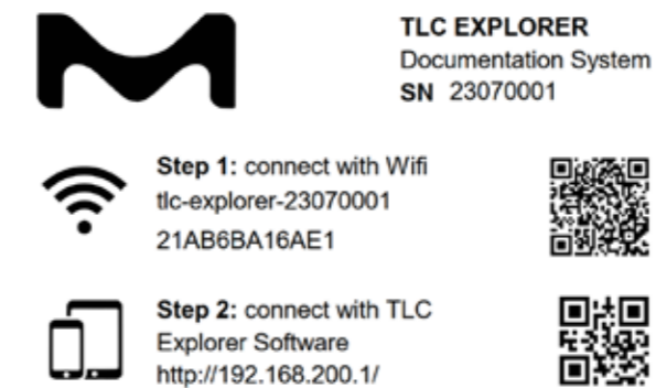
Figure 3.2: Easily connect by scanning these two QR codes on the label of your device
